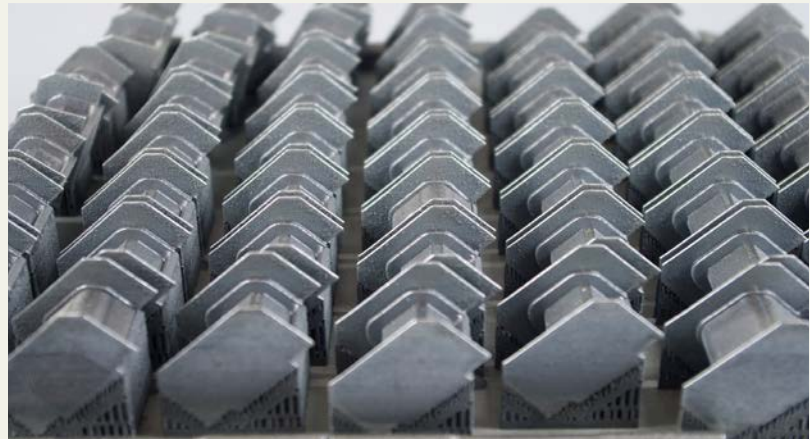
Figure 2: Additive manufactured case A parts: “Edge Insert”
