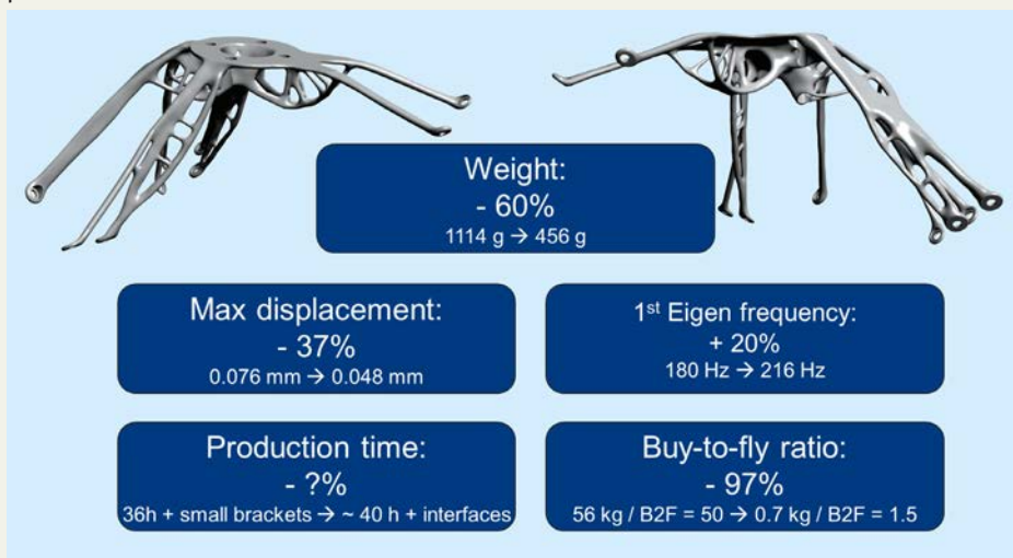
Figure 3: Optimized satellite part and achievements for “Reaction Wheel Bracket”
