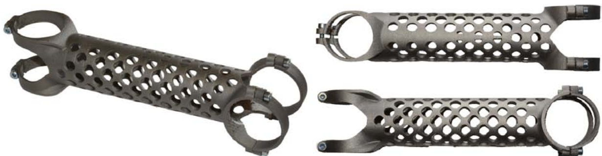
Figure 21: Three different views of additively manufactured bicycle stem with newly introduced crack delay elements
